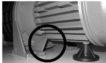
Regularly check the waterproofness! (A leak through a mechanical seal can cause important damages!)
