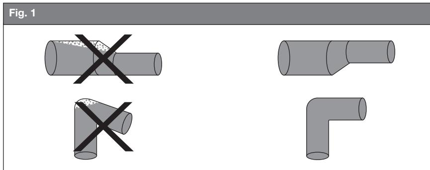
The pipes should be fitted in such a way that any pressure variation caused by temperature changes do not affect the pump.
